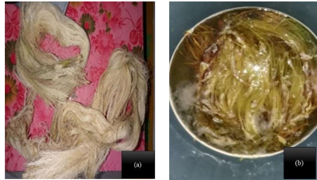
Figure 1: (a) Pineapple leaf fiber, (b) Fiber dipped in NaOH sol.
